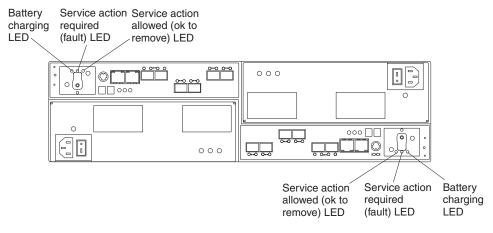
Figure 74. Battery unit LEDs
